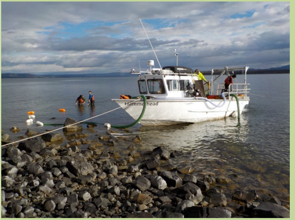
Graph 16: Suction dredge being deployed at Carrington Island to remove LT eggs.
